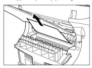
If the jammed paper is badly folded, similar to the folds of an accordion, ease the jammed paper loose and then pull it out of the machine.
